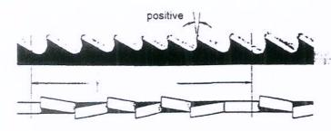
This type of blade is the most suitable for the cutting of section bars and large and thick pipes as well as for the cutting of solid bars at maximum machine capacity. Available pitches: 3-4/4-6.
