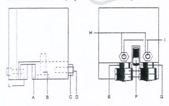
In case the blade needs to be replaced, make sure to always install 0.9mm thick blades for which the blade guide pads have been adjusted. In the case of toothed blades with different thicknesses adjustment should be carried out as follows:
