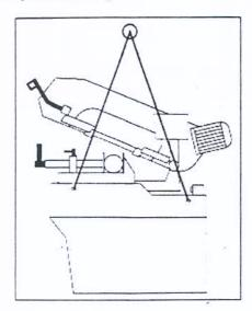
To move the machine, the machine needs to be moved in its own packing, use a forklift truck or sling it with traps as illustrated in the drawing above.
